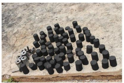
Some of the newly formed charcoal briquettes, produced using waste materials.
